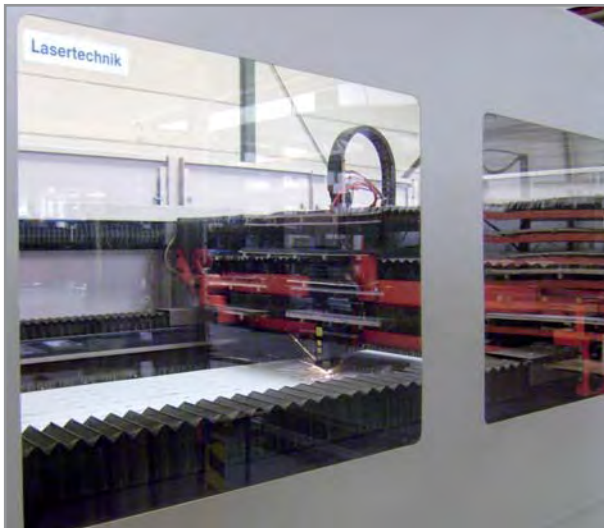
Bellows in operation
